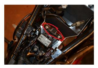
Cable tie Fuel drain pipe to frame as shown
